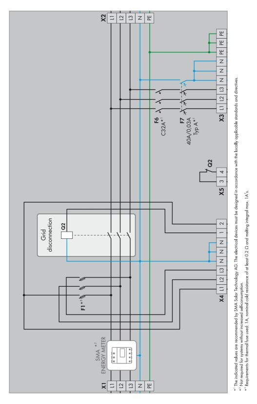
Figure 11: Schematic diagram of the three-phase automatic transfer switch without all-pole disconnection (e.g. for Australia)
