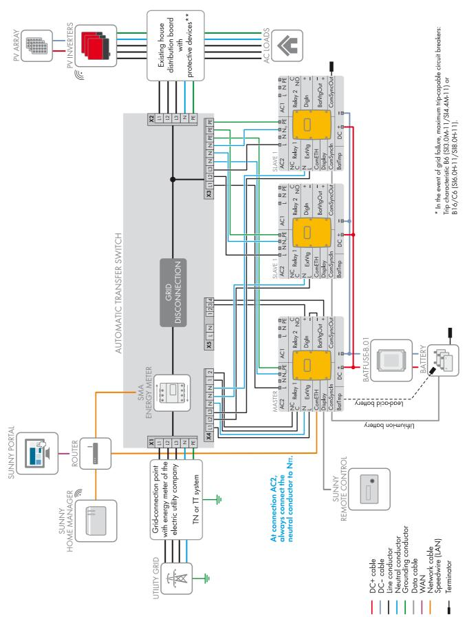
Figure 12: Circuitry overview of a three-phase battery-backup system without all-pole disconnection (e.g. for Australia)
