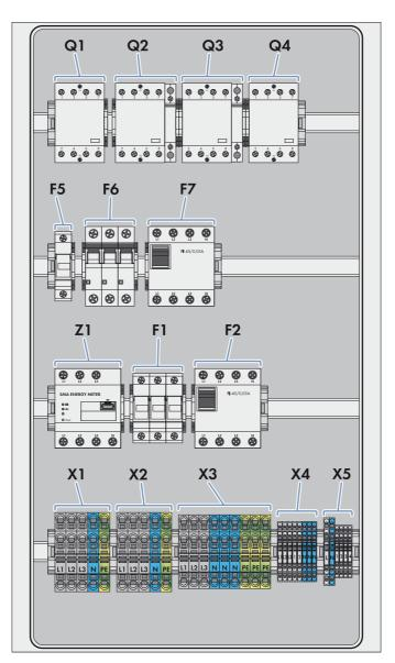
Figure 14: Configuration suggestion for three-phase automatic transfer switch with all-pole disconnection (e. g. for Germany)
