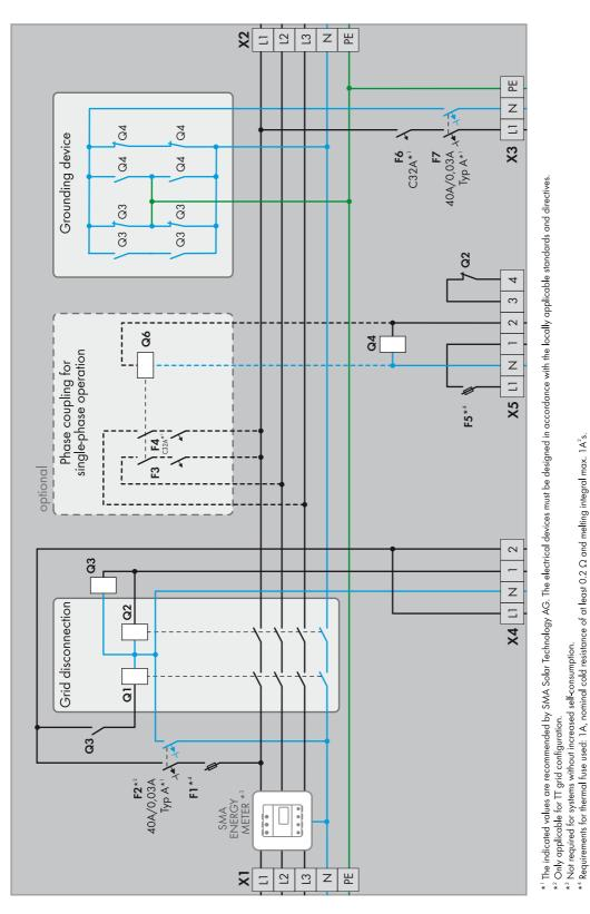
Figure 5: Schematic diagram of the single-phase automatic transfer switch with all-pole disconnection (e.g. for Germany)
