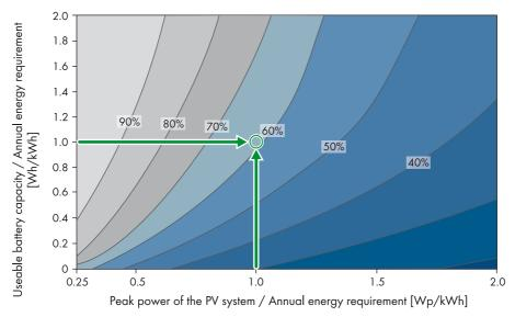
Figure 2: Estimation of self-consumption quota with intermediate storage
